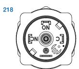
Switch can be wired using either normally open or normally closed configuration. The switch will automatically reset when differential pressure is reduced.
