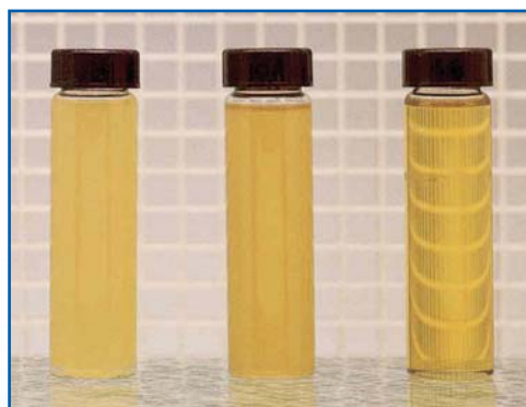
Free water removal in typical turbine oil: bright clear aspect shows absence of free water
